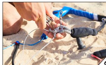
Remove the Trimmer Bracket screw.
